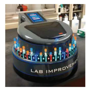
▲ *Lab Improvements' CapTrack is a benchtop device that offers labs an affordable way to automate the recapping of 13mm specimen tubes and manage refrigerated inventory.*
